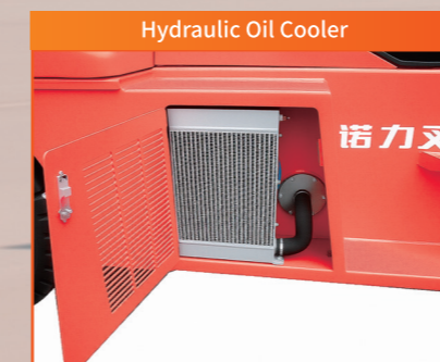
Side-mounted cooler reduces oil temperature.
