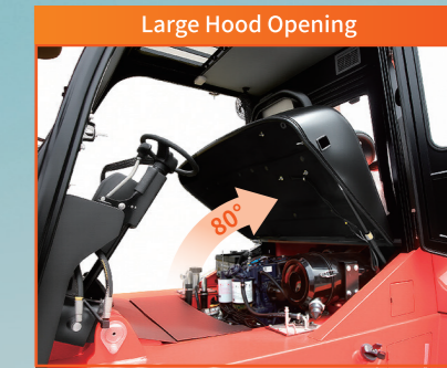
80° engine hood opening for easy access.
