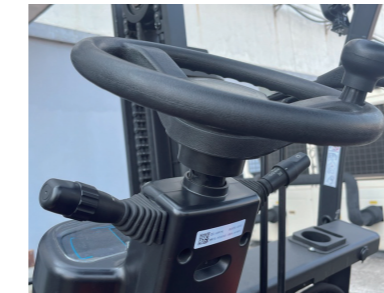
Electro-hydraulic directional switch & multifunction handle (Hydraulic Model).
