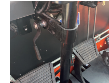
Improved locking mechanism for easy adjustments.
