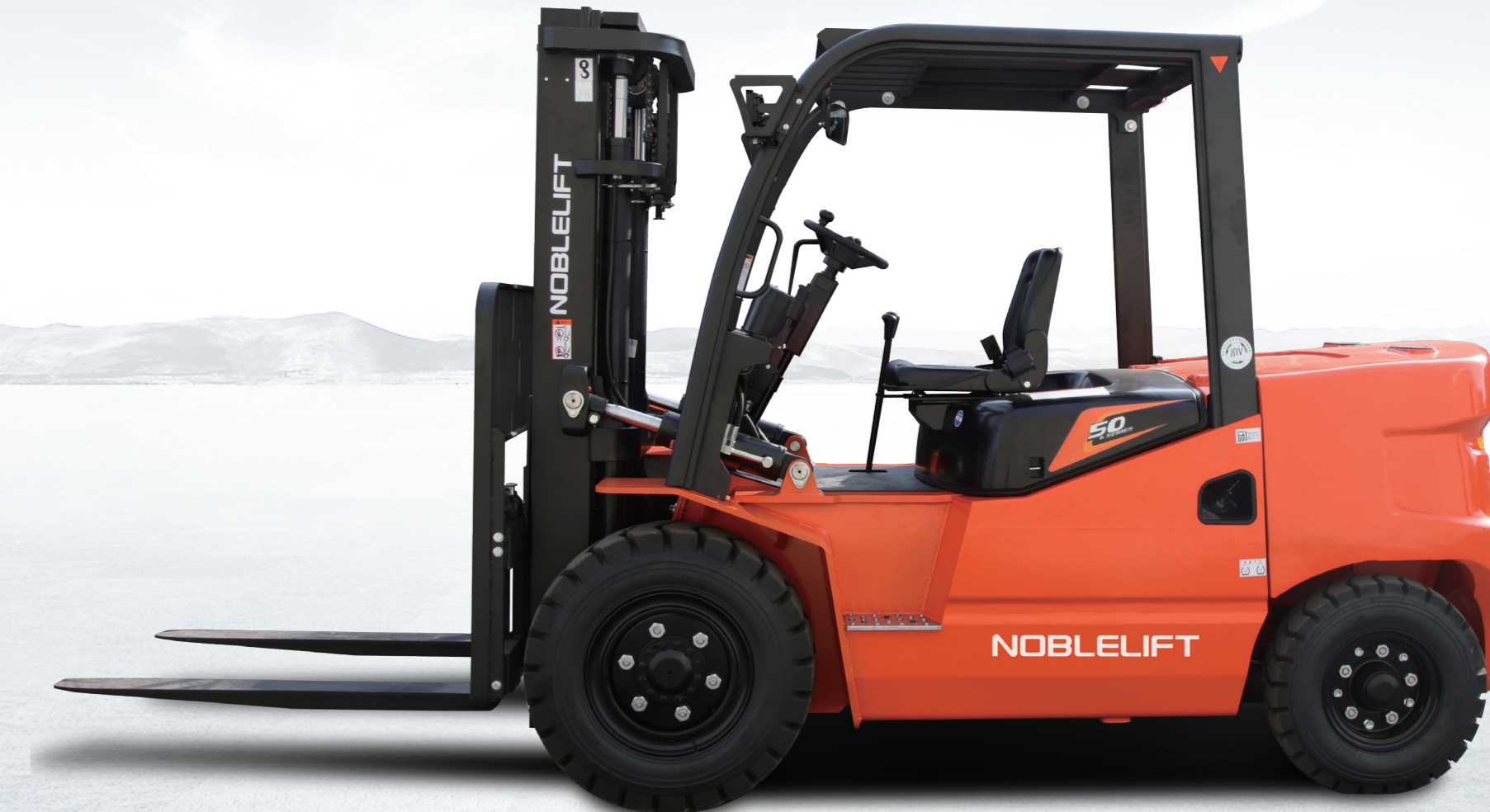
Larger grab handle for easier entry and exit.
