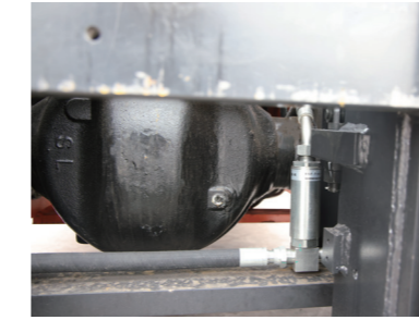
Lift cylinder cushioning for smooth handling.
