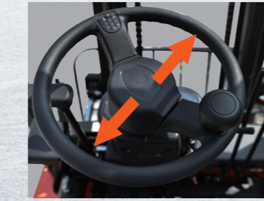
Small-diameter steering wheel for reduced operator effort.
