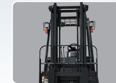
The widened mast provides a better field of vision.
