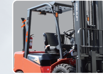
The engine intake pipe uses a high-mounted independent intake, effectively preventing dust from entering.
